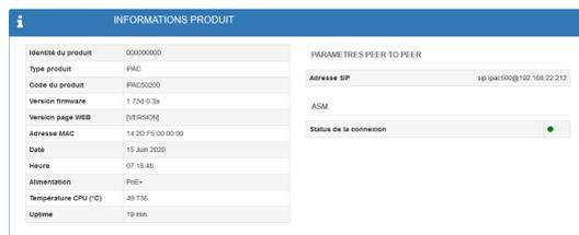
The screenshot shows the 'INFORMATIONS PRODUIT' page. It is divided into two main sections: 'PARAMETRES PEER TO PEER' and 'ASM'. The 'PARAMETRES PEER TO PEER' section includes fields for 'Adresse SIP' (sip:ipac500@192.168.22.212) and 'Statut de la connexion' (Status of the connection), which is currently green. The 'ASM' section is empty. The left side of the page contains a list of product details.
